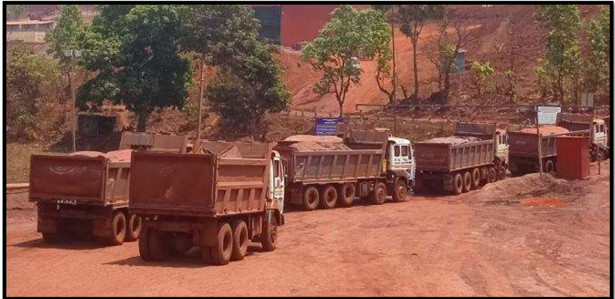
Photo# 8 Ore carrying vehicles covered with Tarpaulin before exit from mine gate
