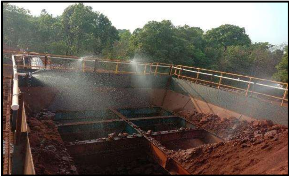
Photo#11 Screen & Crusher plants provided with Dry fog System
